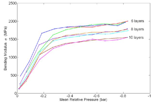
**Figure 2: Bending modulus as a function of pressure and number of layers [3]. The bending modulus stabilizes around -0.4 bar, although the strength of the material can increase for higher vacuum levels. Increasing number of layers reduces the relative stiffness of a Varstiff laminate.**
