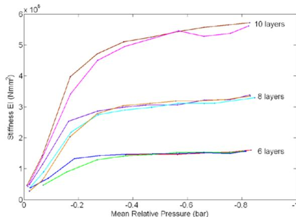
**Figure 3: Sample stiffness as a function of pressure and number of layers. The increase of stiffness is caused by the increase of total laminate thickness and not by an increase of relative stiffness, as shown in Figure 2.**
