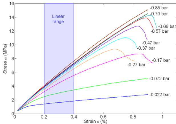
**Figure 1: Stress-strain curves for Varstiff under varying vacuum levels [3]. The stiffness is characterized by the slope of the curve in the blue area, also called the bending modulus of the material, see Figure 2.**
