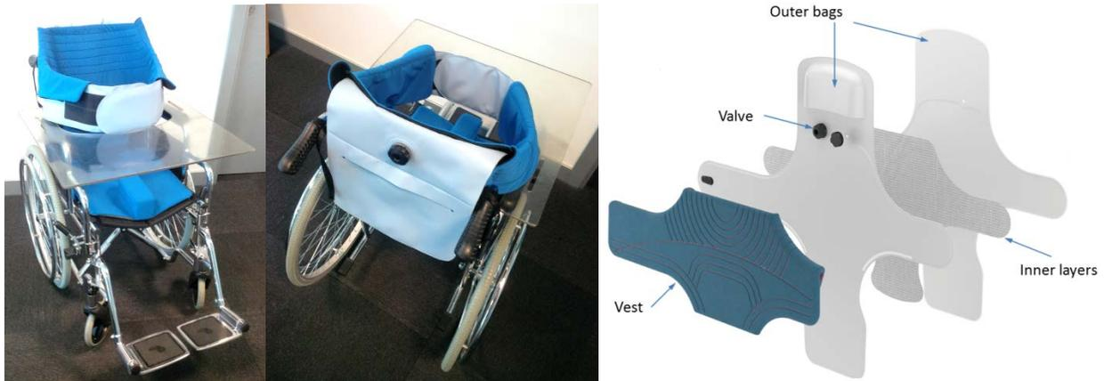
**Figure 4: Final design of the Wheelchair Positioning Device. Left: clearly visible are the “arms” that support the trunk, the pommel cushion to separate the legs, and the blue “comfort vest”. Right: the white bag contains the Varstiff material, and is operated through the black valve placed at the back.**
