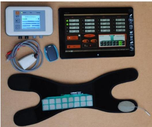
Figure 1. Set-up: INTFES stimulator (Tecnalia Research and Innovation), multiplexer, inertial sensor and garment with multi-pad and PalsPlatinum electrode, tablet PC.
