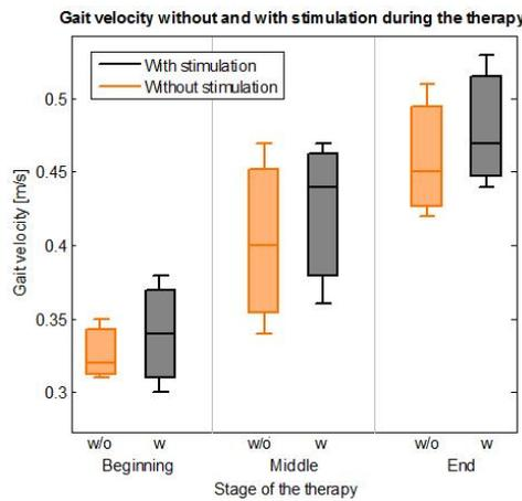
Figure 3. Gait velocities during 10 m test with (grey boxes) and without (orange boxes) aid of the FES at the beginning, middle and end of the therapy.
