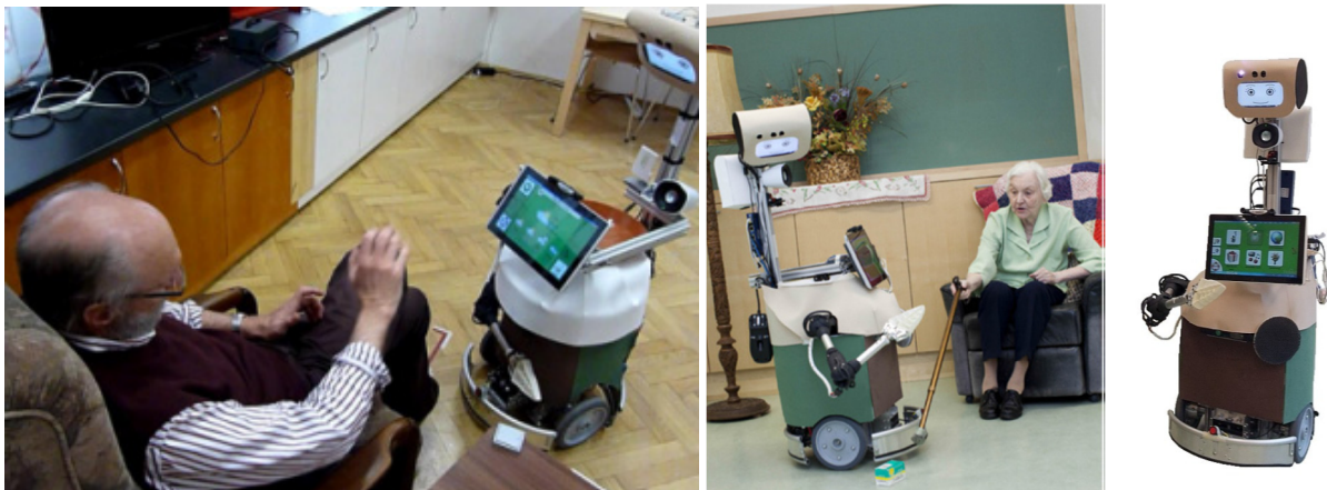
Fig. 2: Multimodal UI on the assistive robot Hobbit (Prototype 1) during user Interaction scene in lab (left) and during user trials (middle). Front view first prototype of Hobbit robot (right).
