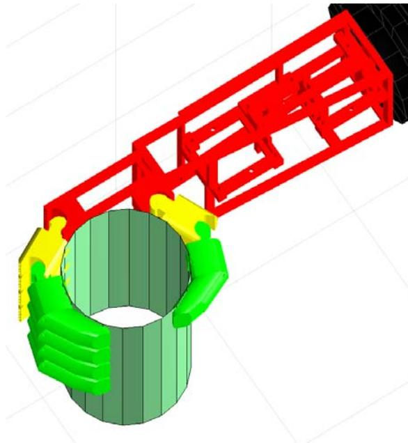
**Figure 4: KUKA KR3 grab a cylinder**
