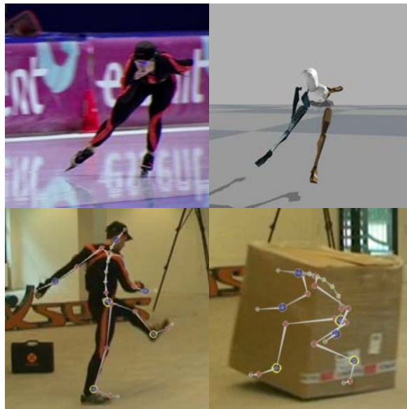
Figure 1 Examples of inertial motion capture. Upper left: olympic and world champion speed skating Ireen Wüst wearing an inertial motion capture suit with 17 inertial sensors. Upper right: graphical representation of the estimated position and orientation of the body segments. Lower left and right: experiment showing that line of sight visibility is not necessary for inertial motion capture.
