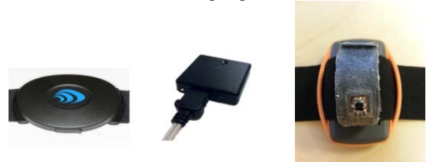
Figure 2 (a) Chest Unit with elastomer electrodes (b) Dual channel EMG unit. (c) IsenseU sensor unit
