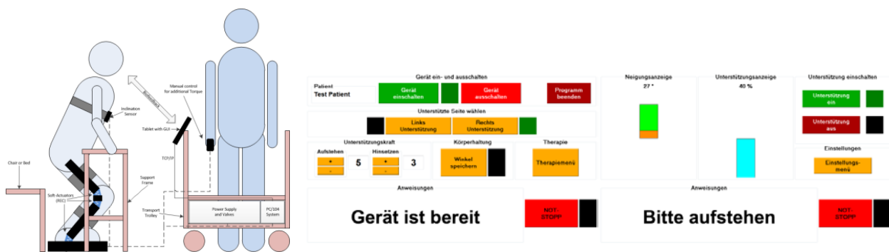
Fig. 1: Sit-to-Stand trainer: Conceptual design and Graphical User Interface with settings and therapy menu.
