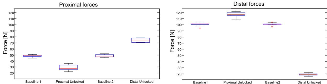
Figure 3: The force amplitudes of one subject measured in the human exoskeleton interface underneath the cuffs. The proximal forces were recorded underneath the proximal cuff, the corresponding distal forces underneath the distal cuff.
