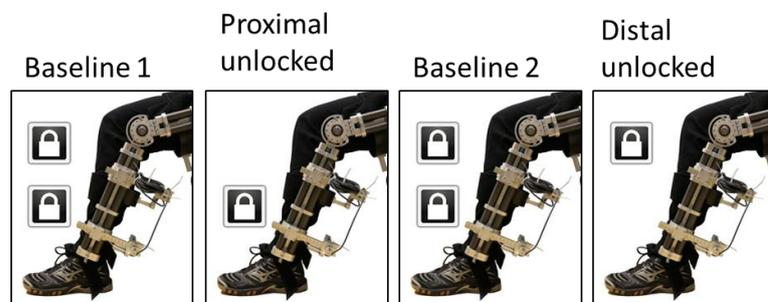
Figure 2: The experimental setup and protocol, the subjects were in a seated position and conducted 15 isolated knee movements from  $0^\circ$  to  $90^\circ$  flexion in each condition. The second baseline measurement was conducted to ensure that the setup was not altered. The forces were measured in the cuff attachment parallel to the shank exoskeleton structure.
