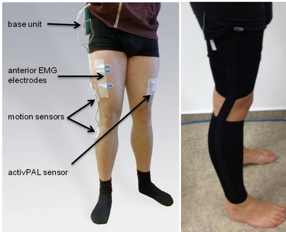
**Figure 1:** Monitoring system components without orthosis (left) and integrated into a soft orthosis (right).
